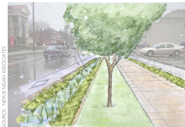
Figure 2-8: By utilizing a more efficient site design, the wasted space in the street example above can easily be converted into conventional landscaping or be used for stormwater facilities. This retrofit opportunity also includes space for a bike lane.
