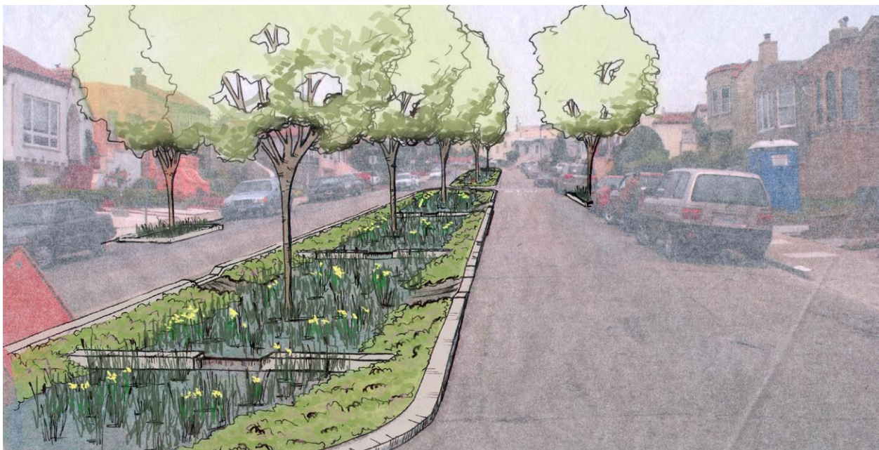
Figure 4-25: RETROFIT OPPORTUNITY: The same residential street retrofitted with a stormwater median swale. Note the illustrated check dams and weirs that help terrace the steep grade of the street and help control the desired water retention depth.
