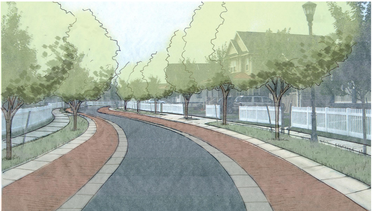
Figure 4-15: RETROFIT OPPORTUNITY: The same residential street retrofitted with pervious paving in the parking zone.
