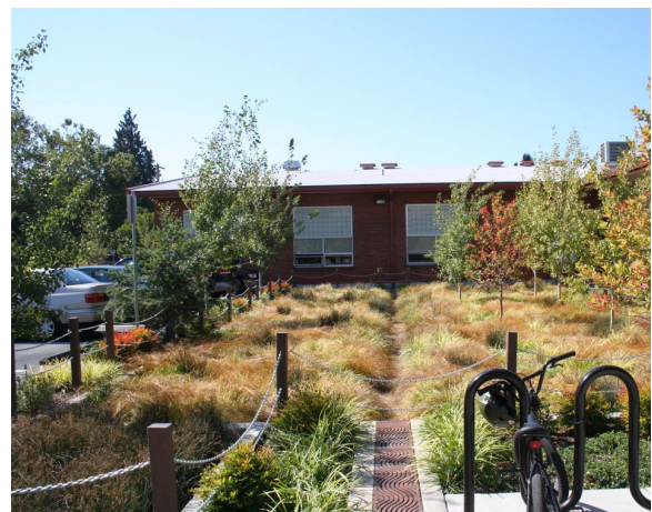
Figure 2-78: This rectangular rain garden area receives runoff from both a parking lot and the building's rooftop.
