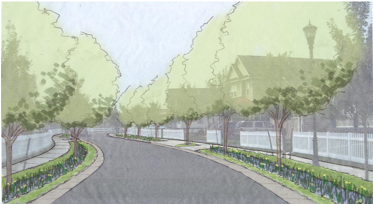
Figure 4-17: RETROFIT OPPORTUNITY: The same residential street using vegetated swales within the street's planting strips.
