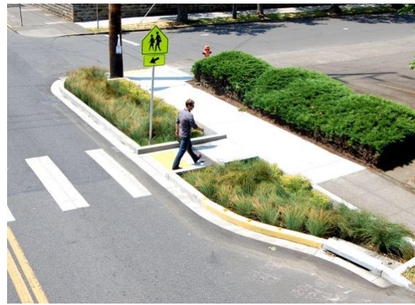
Figure 2-88: Accessible pedestrian ramps can also be integrated into the design of stormwater curb extensions.
