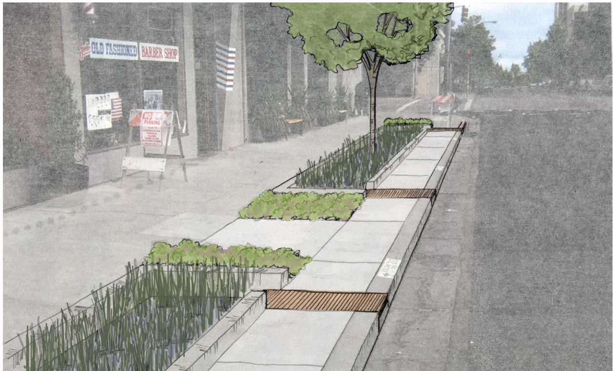
Figure 4-33: RETROFIT OPPORTUNITY: The same commercial street retrofitted with stormwater planters.
