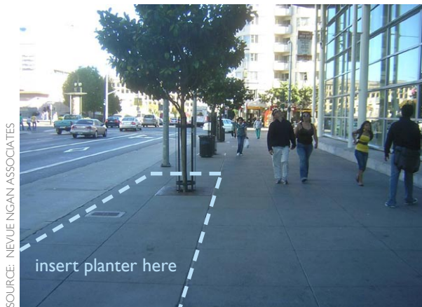
Figure 2-61: Planters can be retrofitted on urban streets with overly wide sidewalk zones. Dashed lines show where a planter could be added.
