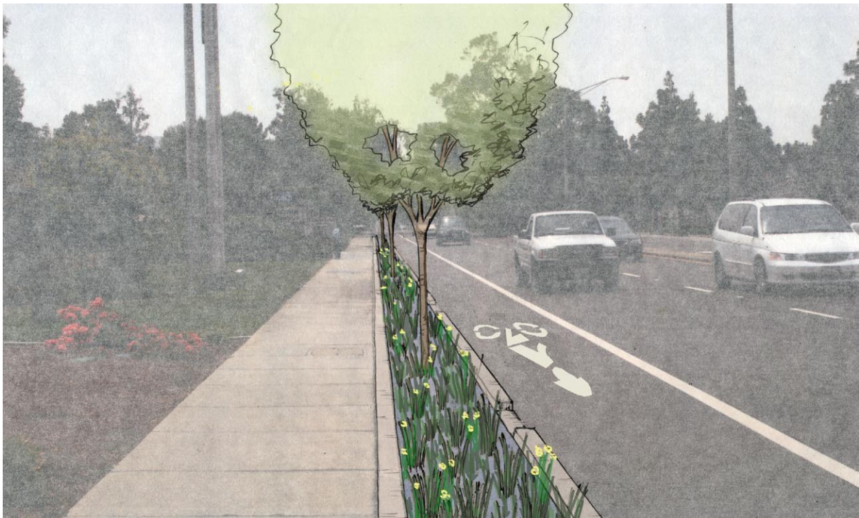
Figure 4-46: RETROFIT OPPORTUNITY: The same street retrofitted with a green gutter along the existing asphalt shoulder.
