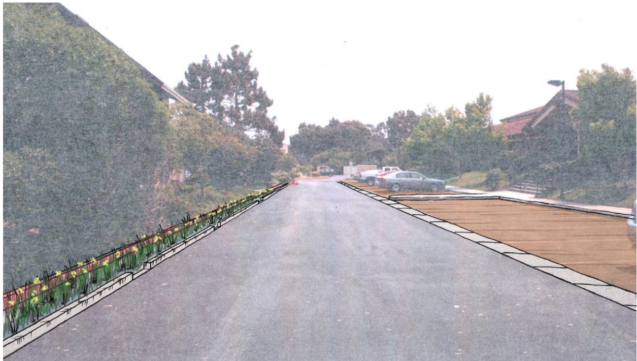
Figure 4-64: RETROFIT OPPORTUNITY: The same parking lot retrofitted with a green gutter and pervious paving in the parking stalls.
