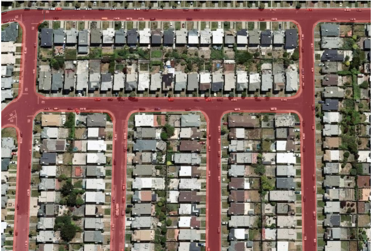
Figure 3-5: The red areas superimposed on this aerial photo illustrate the impervious street area that generates runoff from high-density residential streets.
