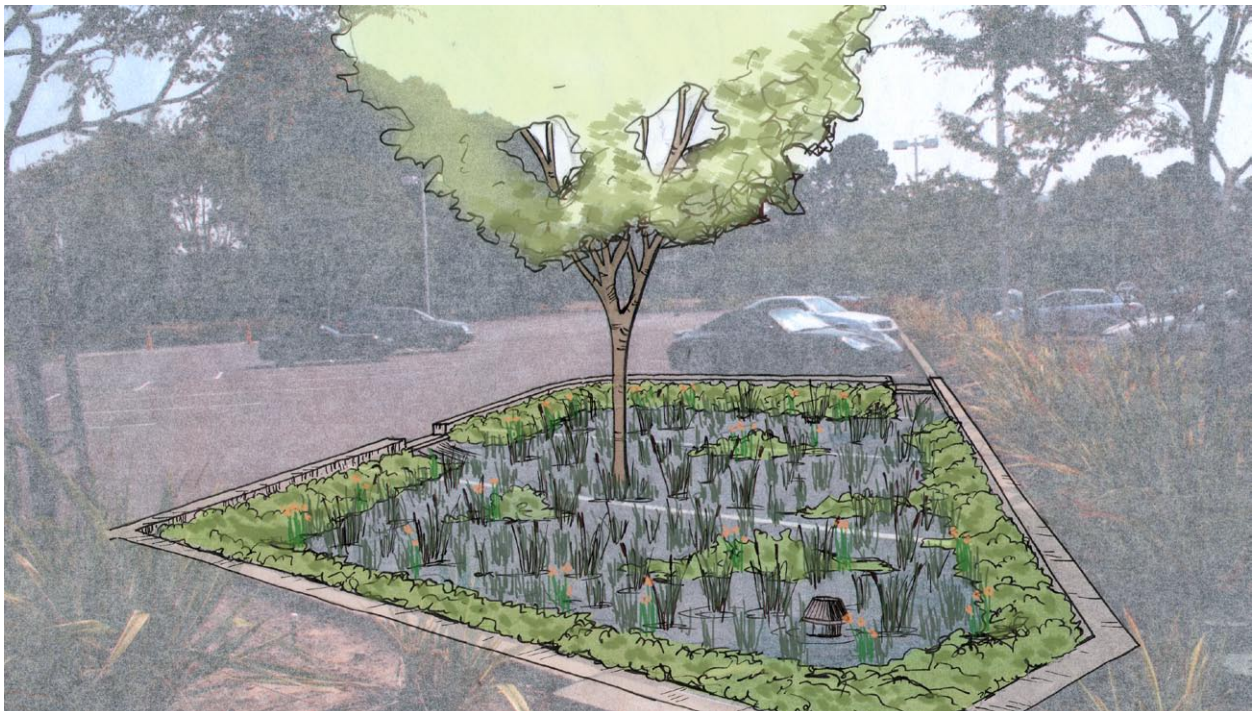
Figure 4-55: RETROFIT OPPORTUNITY: The same parking lot retrofitted with a stormwater planter. Notice that this stormwater planter is located near the existing drainage inlet.
