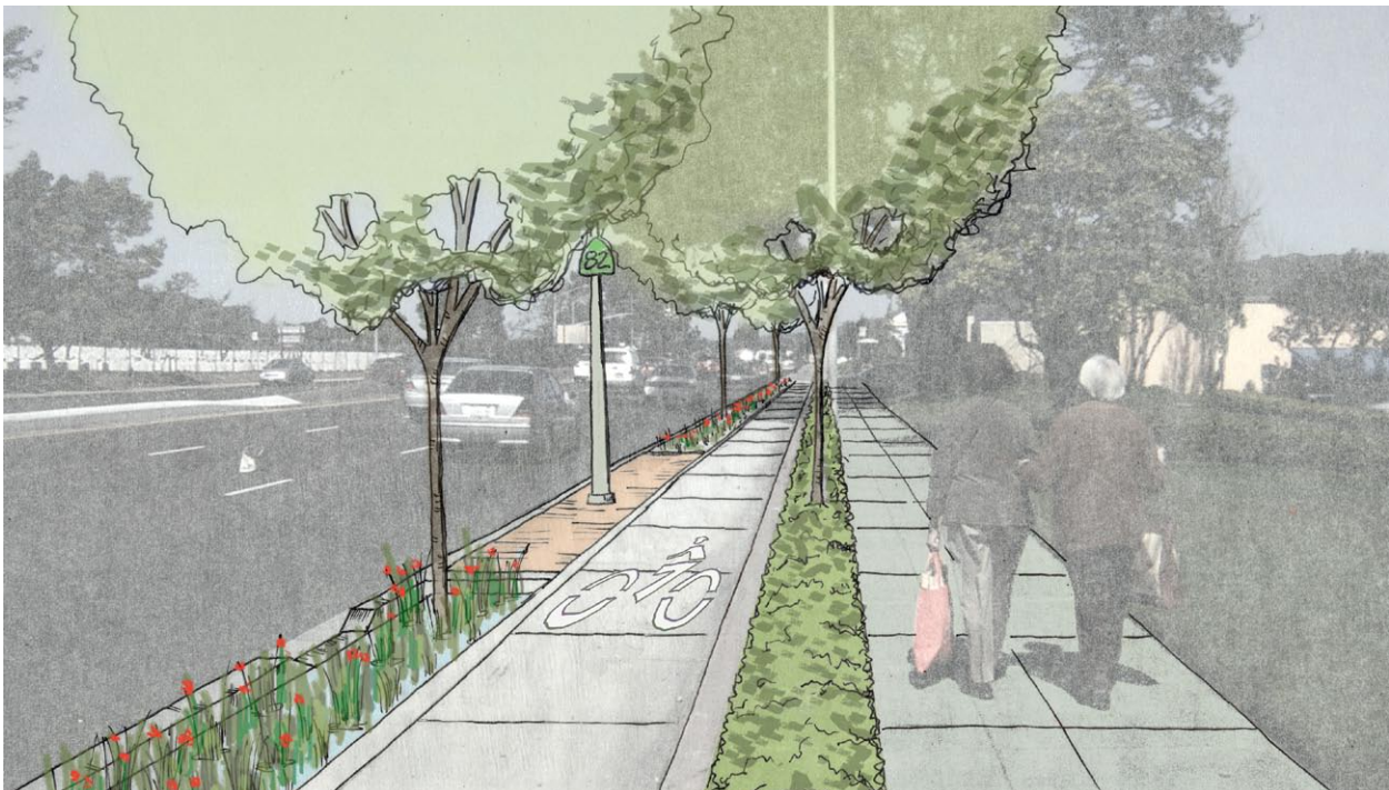
Figure 4-50: RETROFIT OPPORTUNITY: The same street retrofitted with a series of stormwater planters, a separated bike path, and additional street trees.
