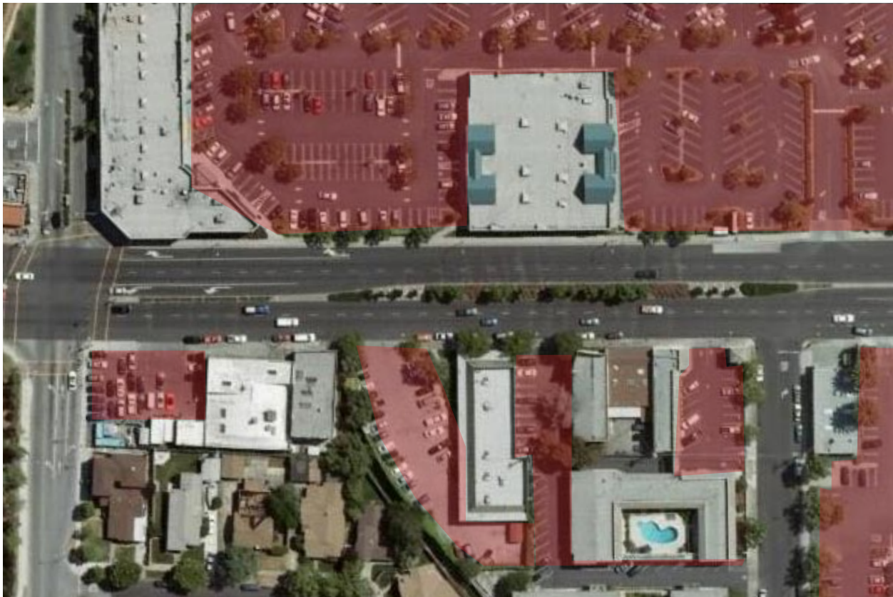
Figure 3-11: The red areas superimposed on this aerial photo illustrate the impervious parking lot area that generates runoff from small and large parking lots.
