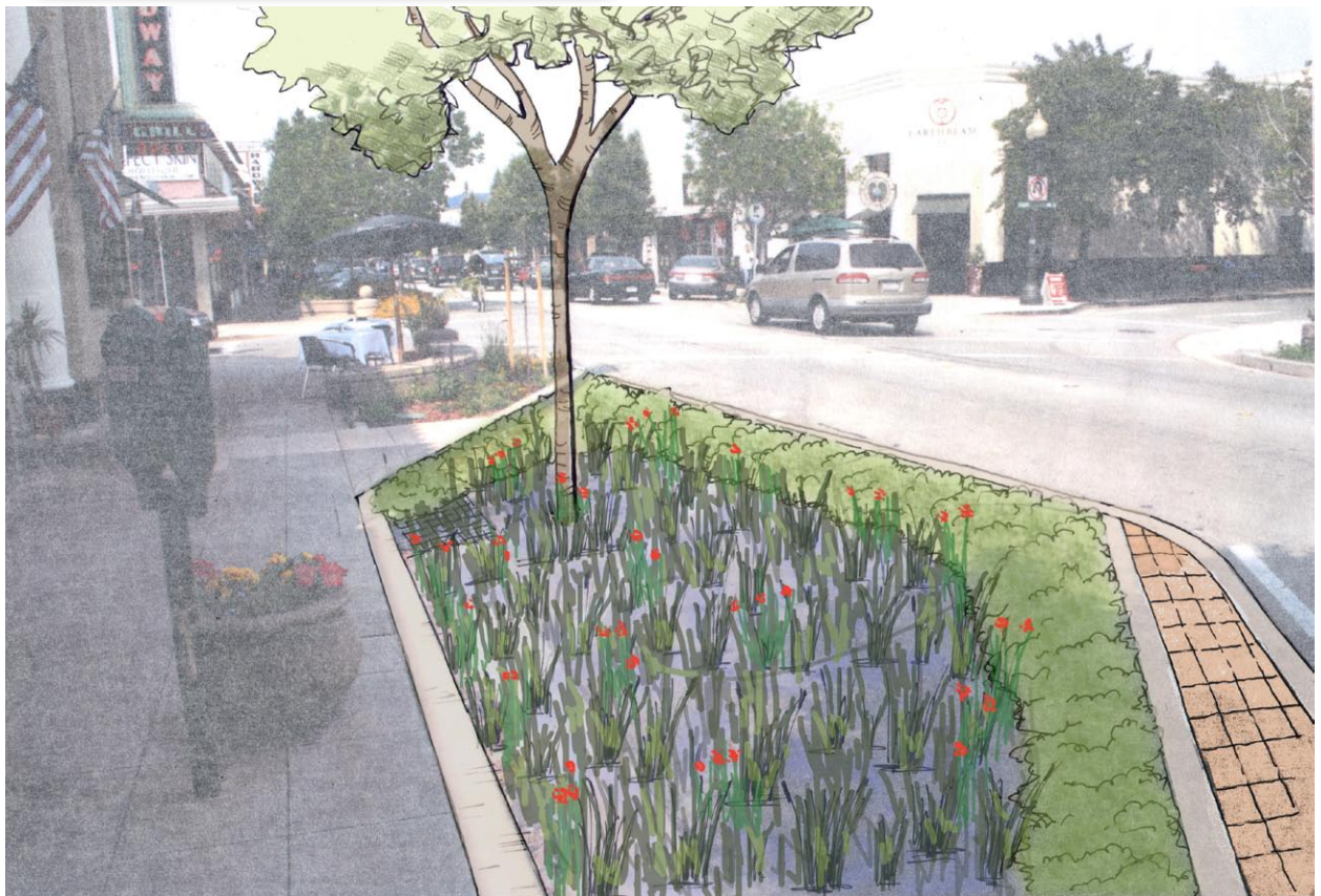
Figure 4-38: RETROFIT OPPORTUNITY: The same commercial street with two angled parking stalls converted into a stormwater curb extension.
