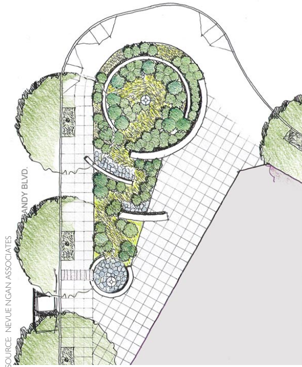
Figure 5-1: The conceptual design of a rain garden on Sandy Boulevard in Portland, Oregon.
