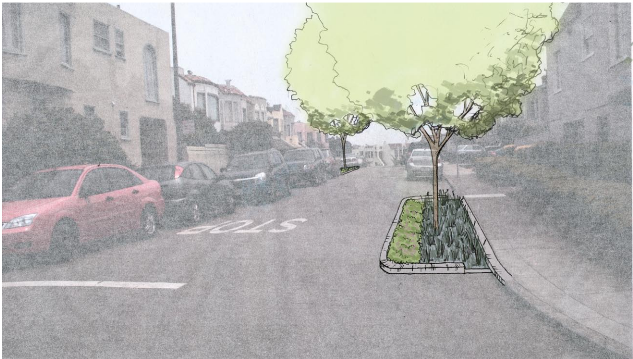
Figure 4-22: RETROFIT OPPORTUNITY: The same residential street using short curb extension in between driveways.
