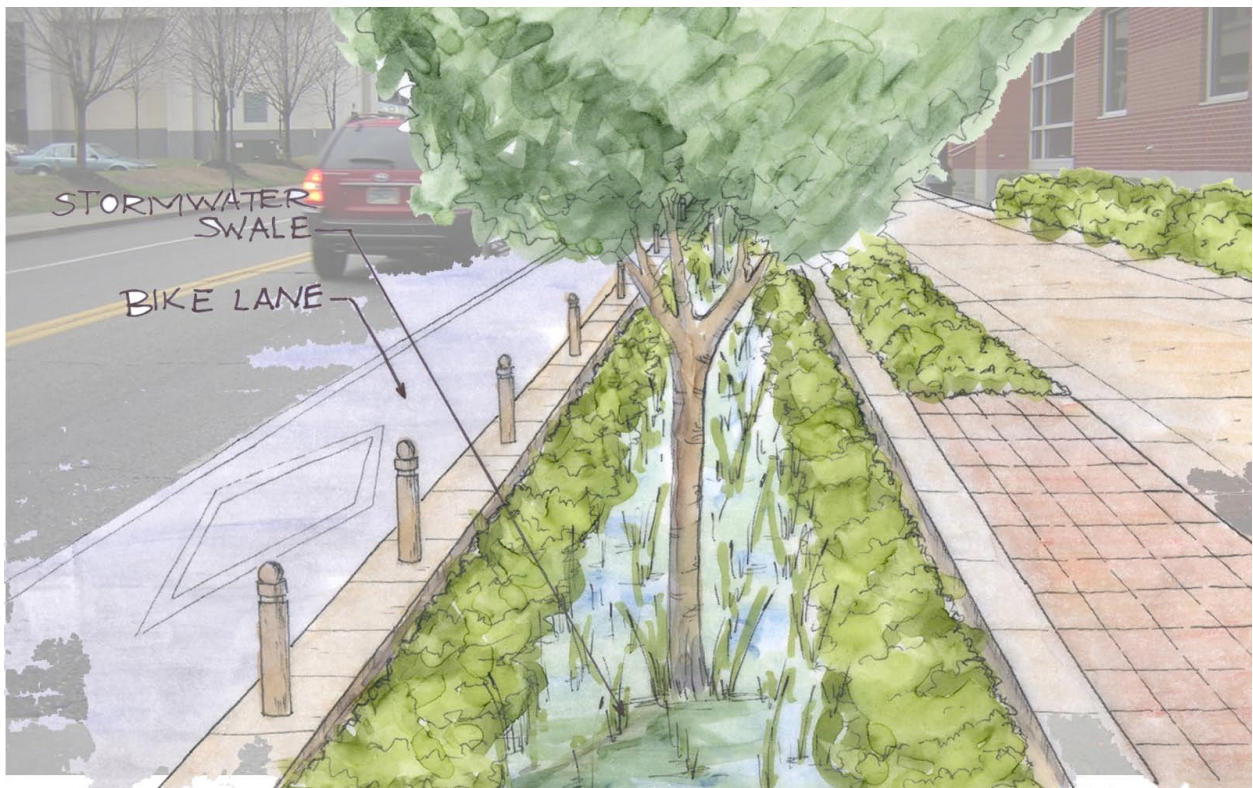
Figure 4-36: RETROFIT OPPORTUNITY: The same street without one traffic lane and retrofitted with a “curbless” street, vegetated swale, and bike lane.
