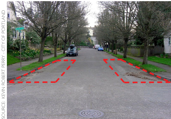
Figure 2-83: Parking zones on residential streets are prime candidates for stormwater curb extension retrofits. Dashed lines show where a stormwater curb extension could be added.
