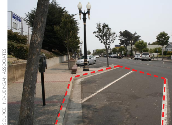
Figure 2-82: Angled parking stalls in downtown streets can be converted into stormwater curb extensions and would provide more of a balance between landscaping and parking. Dashed lines show where a stormwater curb extension could be added.
