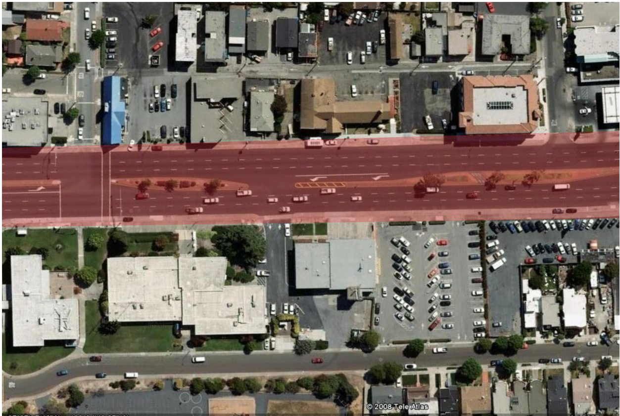
Figure 3-9: The red areas superimposed on this aerial photo illustrate the impervious street area that generates runoff from a multi-lane arterial street.
