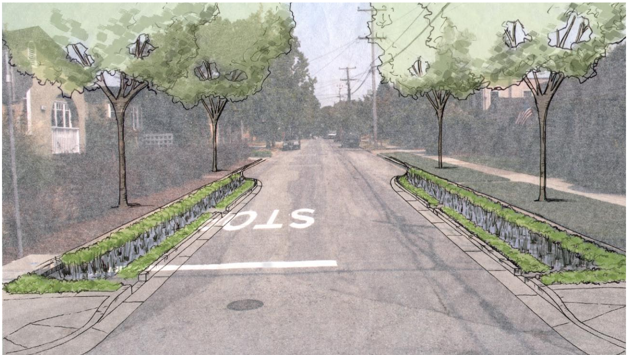
Figure 4-6: RETROFIT OPPORTUNITY: The same residential street retrofitted with stormwater curb extensions, as well as additional street trees.
