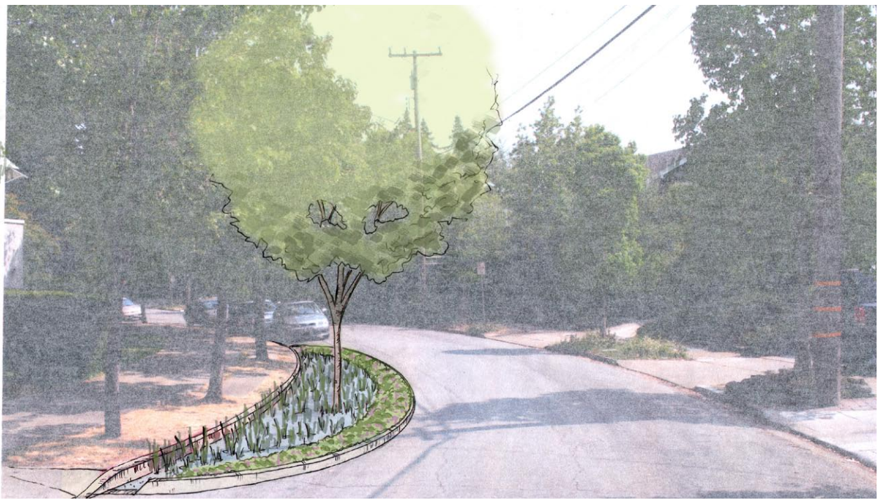
Figure 4-9: RETROFIT OPPORTUNITY: The same residential street retrofitted with mid-block stormwater curb extension, as well as an additional street tree.
