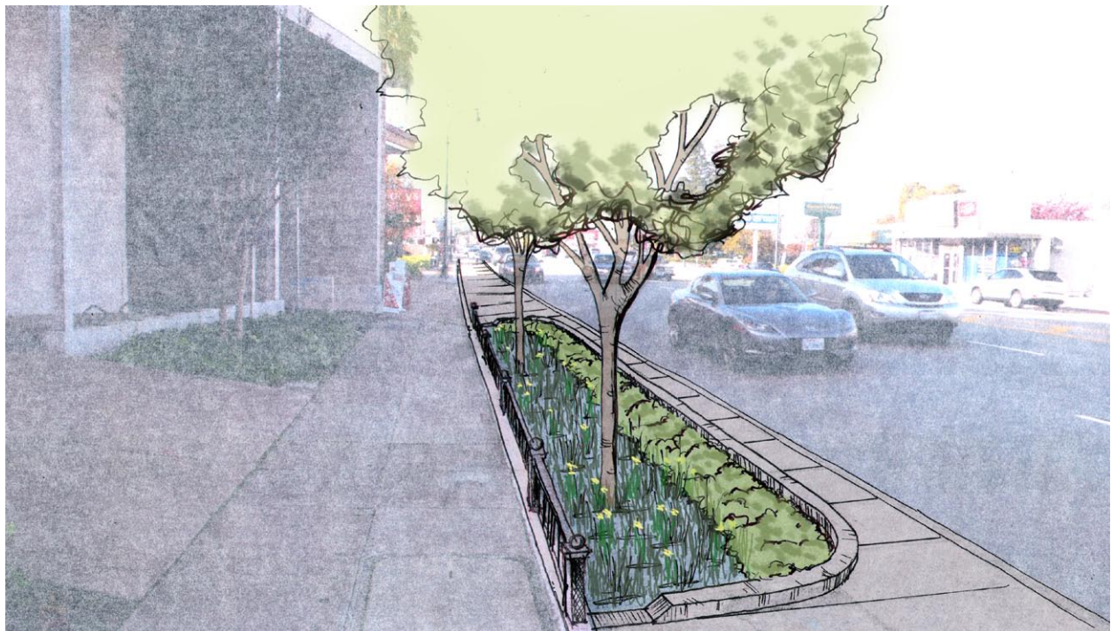
Figure 4-48: RETROFIT OPPORTUNITY: The same street retrofitted with a stormwater curb extension in the parking zone. In this example a low-profile railing has also been added to the streetscape.
