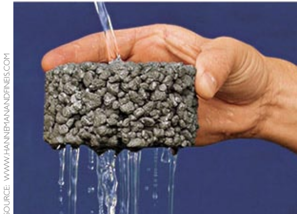
Figure 2-40: Pervious concrete allows water to pass through pore spaces within the aggregate.
