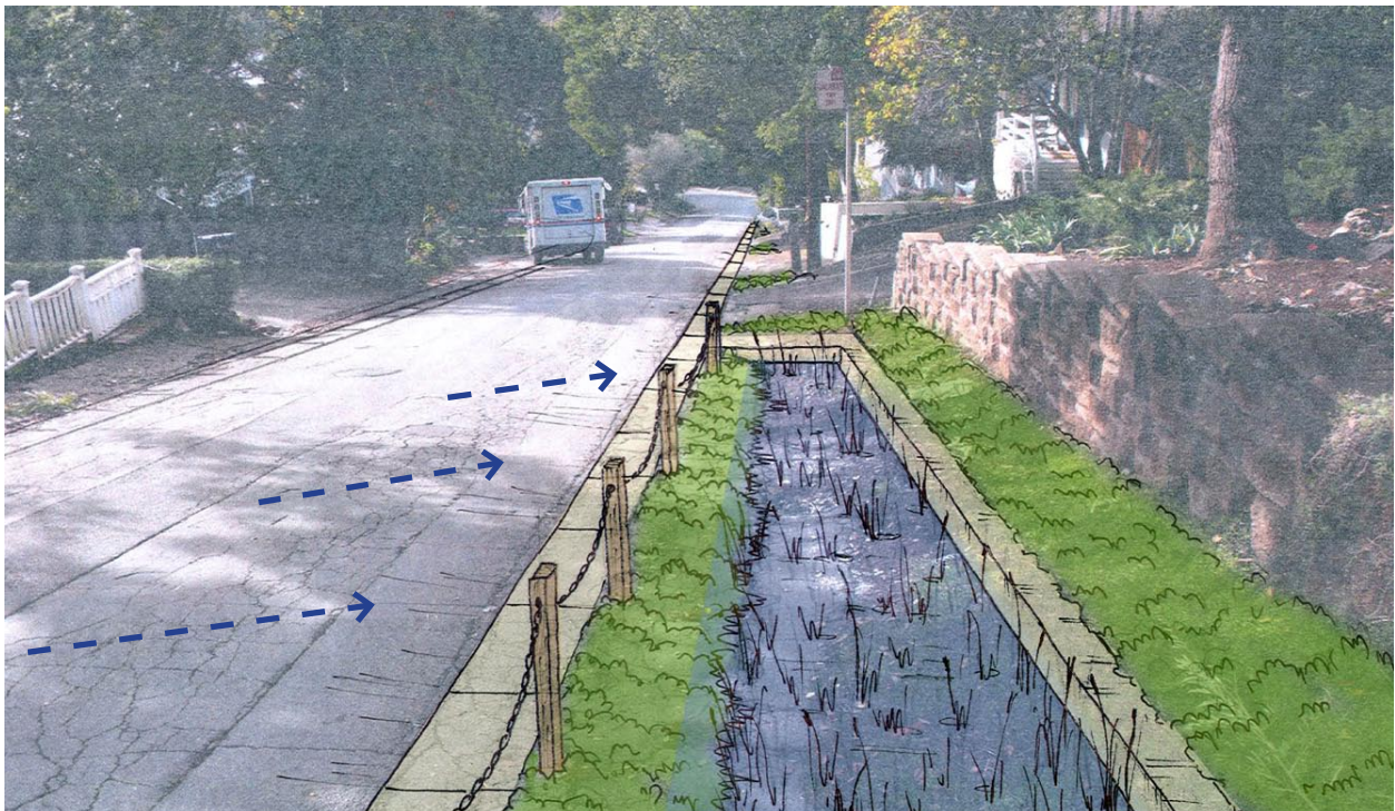
Figure 6-28: An early concept rendering showing how Design Option #2 would function with a vegetated swale/planter along the west side of Holly Road.
