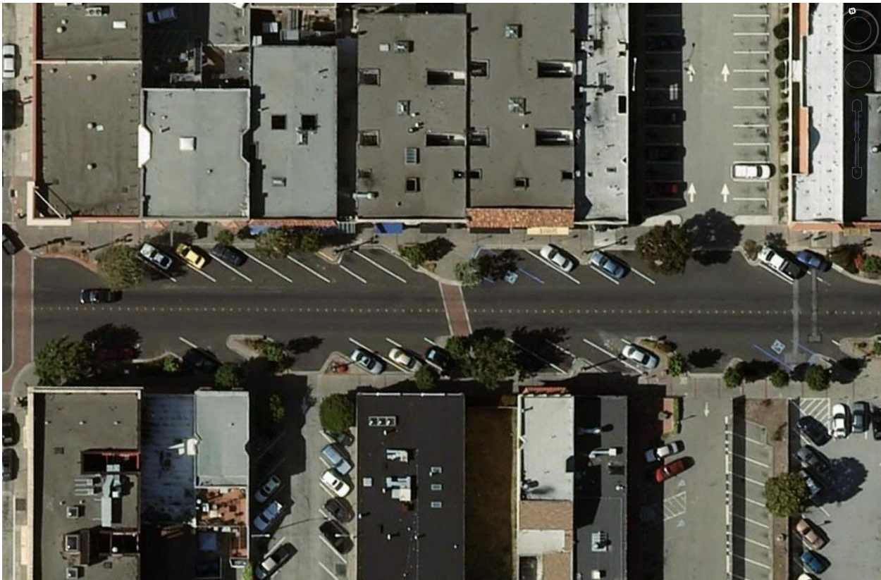
Figure 2-13: An aerial view of a commercial main street using 30 degree angled on-street parking. Notice how much space is wasted at the back end of each oversized parking stall. Also notice the narrow the sidewalk zone.
