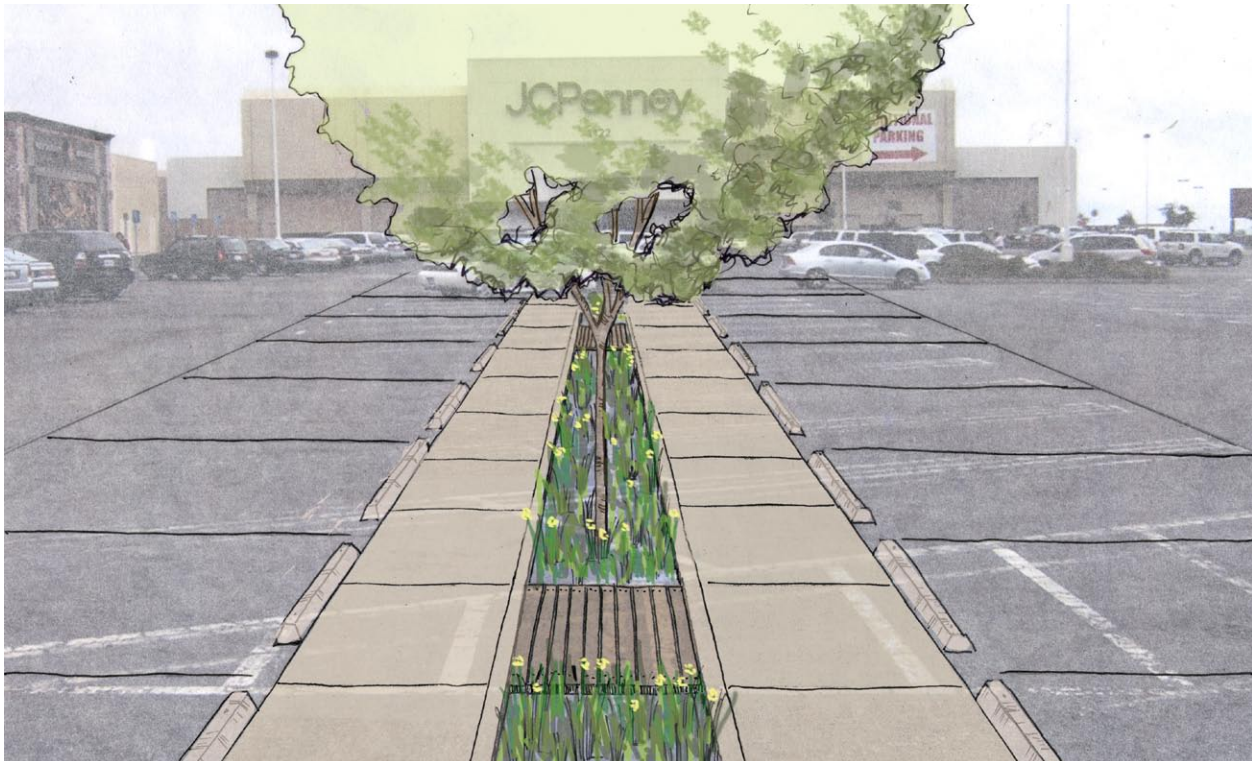
Figure 4-61: RETROFIT OPPORTUNITY: The same parking lot retrofitted with a stormwater planter/vegetated swale. Notice the sidewalk zones and dedicated crossings to allow for adequate pedestrian circulation.
