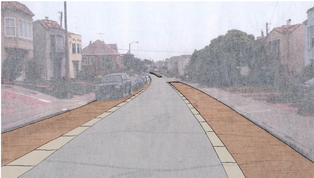
Figure 4-19: RETROFIT OPPORTUNITY: The same residential street retrofitted with pervious paving in the parking zone of the street.
