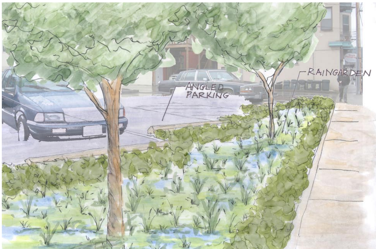
Figure 4-53: RETROFIT OPPORTUNITY: The same parking lot retrofitted with a vegetated swale/planter.
