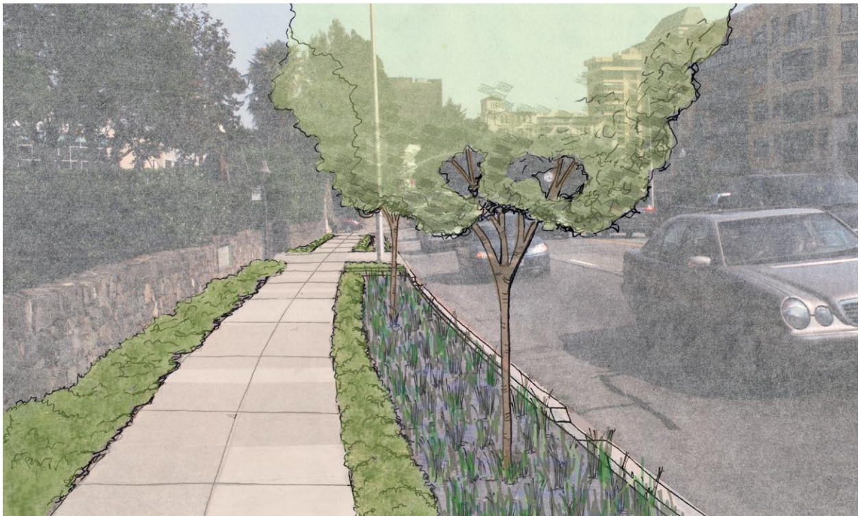
Figure 4-43: RETROFIT OPPORTUNITY: The same street retrofitted with a vegetated swale within the existing planting strip.
