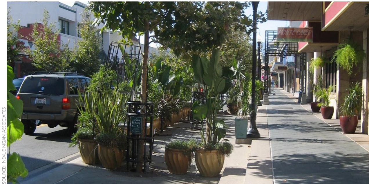
Figure 2-22: This innovative example in Mountain View, CA boldly greens the street with street trees and moveable planters. The planters can be placed in the parking zone to create additional space for tables and seating or can be removed to maintain on-street parking. This is an excellent example of balancing parking spaces with landscape and people space.
