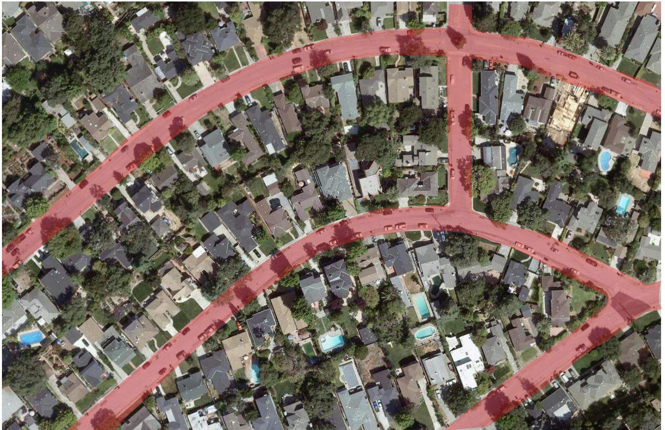
Figure 3-3: The red areas superimposed on this aerial photo illustrate the impervious street area that generates runoff from low-density residential streets.
